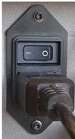
Figure 4-2 Main power switch and cable
