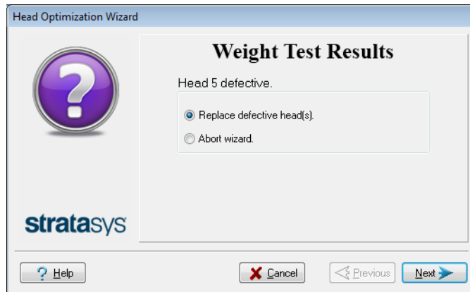
Figure 4-76 Defective print heads found
