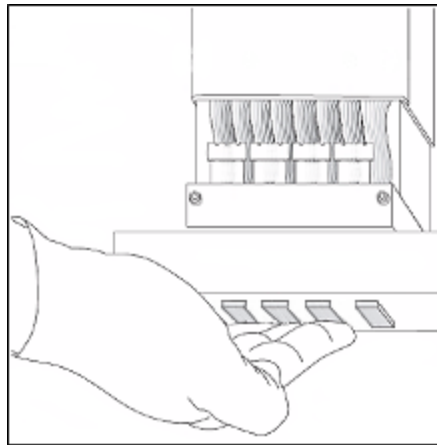
Figure 4-91 Checking the level of the new head
