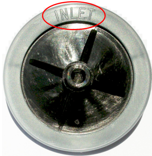
Figure 4-132 INLET side of the filter
